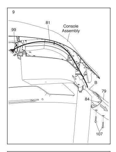
Remove the two #8 x 1 1/4" Screws (107) and slide the Right Handrail Cover (80) back about 1 in. The Screws will be reattached in step 16. Note: It is not necessary to move the Right Handrail Insert (85).
